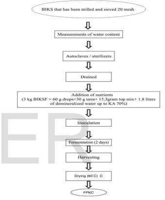
Picture 1. BIS fermentation process flow diagram with *Candida utilis.*
